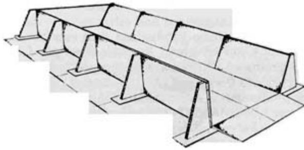
**Figure 2.** Stockpiles With Permanent Ground Liners
